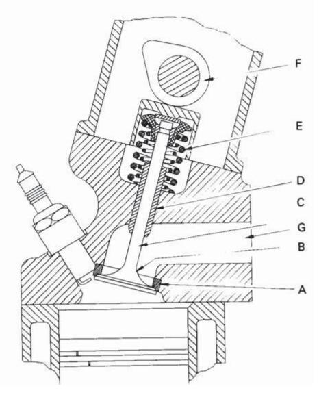
Poppet valve is spring loaded closed, and pushed open by cam action at proper time in cycle. Most automobile engines and other reciprocating engines use poppet valves. Much less common are sleeve valves and rotary valves. Components include: (A) valve seat, (B) head, (C) stem, (D) guide, (E) spring, (F) camshaft, (G) manifold
