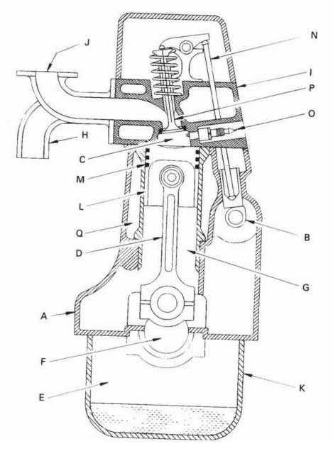
**Figure 1-15** Cross-section of four-stroke cycle S1 engine showing engine components; (A) block, (B) camshaft, (C) combustion chamber, (D) connecting rod, (E) crankcase, (F) crankshaft, (G) cylinder, (H) exhaust manifold, (I) head, (J) intake manifold, (K) oil pan, (L) piston, (M) piston rings, (N) push rod, (0) spark plug, (P) valve, (Q) water jacket.
